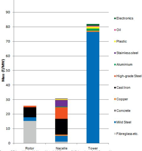
Figure A3: Composition of a Geared Wind Turbine
